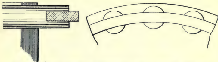
FIG. 107.—Typical methods of fastening end rings to circular Rotor Bars.
